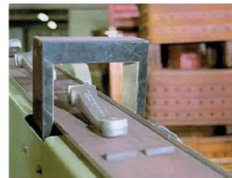
Fig. 1: Example of forging parts inspection
